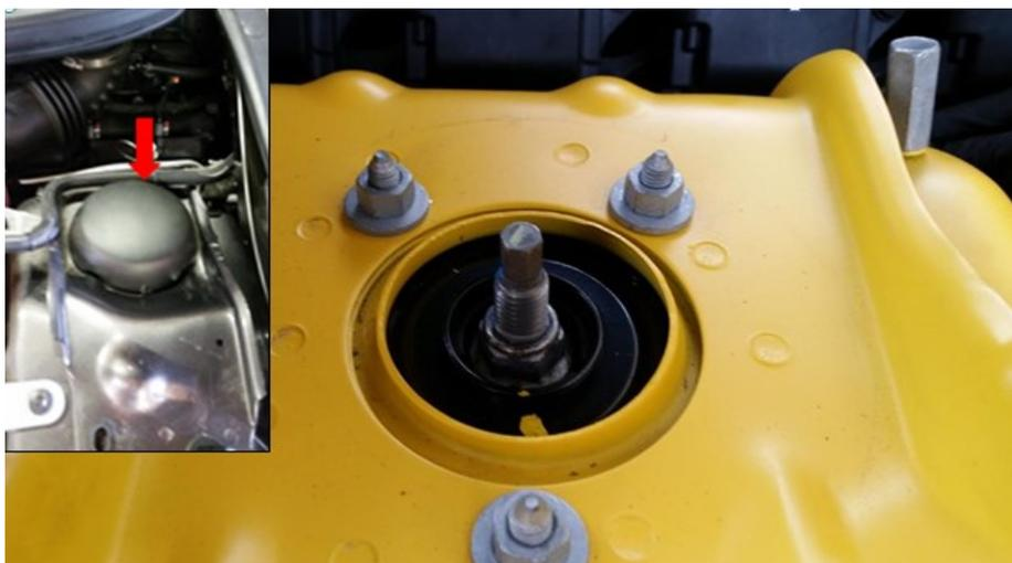
1. Locate the production strut caps and remove with a plastic trim tool. Verify there are 7-8 threads on the strut tower to install the new MOPAR Strut Caps.
