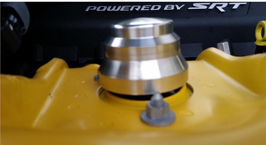
4. Carefully thread the cap onto the shock tower and hand tighten until snug. The gap between the strut frame and the Strut Tower Cap should be similar to image. Additional Washers are provide for adjustment and variation.
